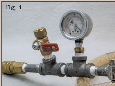
Regardless of your vacuum pump setup and plumbing, the widely available Milton fitting will make a proper connection.
