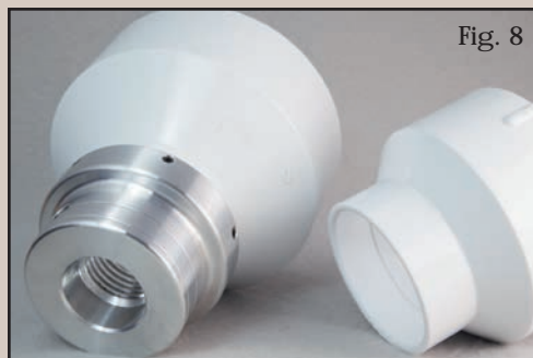
You can buy several hubs and make as many vacuum chucks as you need or you can change PVC fittings as needed.
