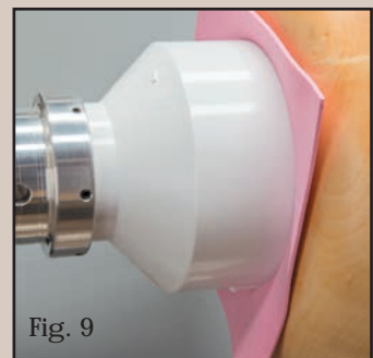
I find a very workable seal can be made with a piece of 2mm craft foam without any permanent attachment to the chuck.
