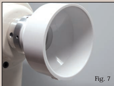
With the PVC fitting seated and setscrewed in place, the vacuum chuck is ready for use.
