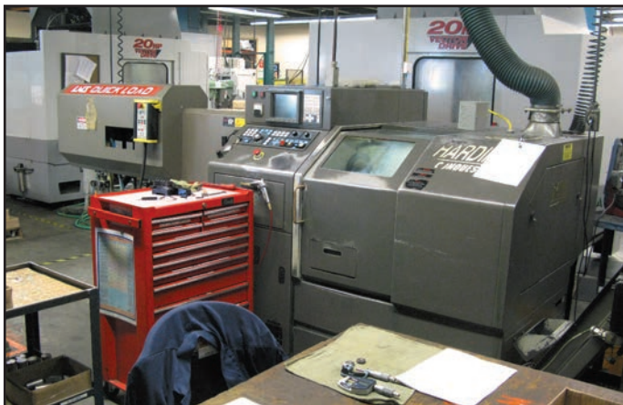
Fig. 8. With successful products selling in the one to two thousand per year range, the key to Veritas manufacturing is flexibility. CNC equipment, whether lathes, mills, or others, makes low-number manufacturing runs practical.
