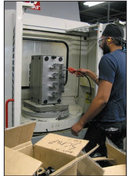
Fig. 10. CNC machining centers using tool magazines and tombstones make mixed-lots of work possible. The various manufacturing runs can vary from a few to hundreds, but it is always still a modest number compared to high-volume operations.
