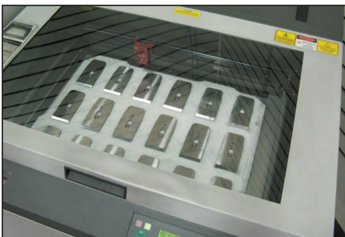
Fig. 15. With all the various part numbers that need to be permanently indicated on the predominately metal parts, a marking laser is the only way to go. The logo and part number are inscribed and also the day/date code of manufacture.
