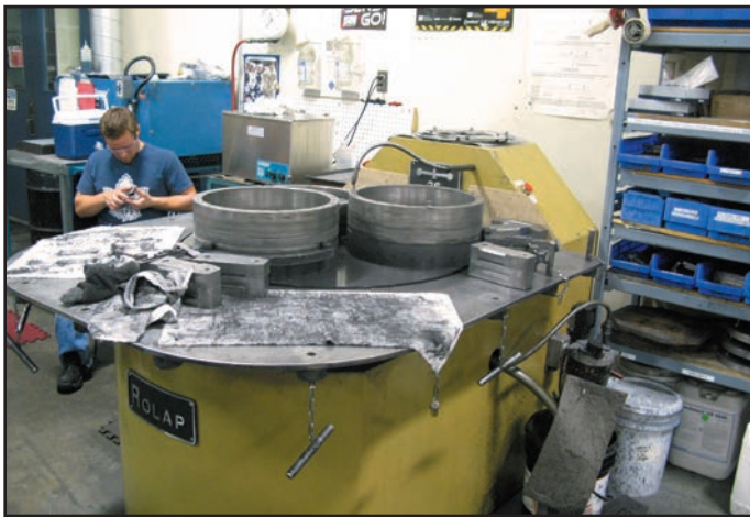
Fig. 14. How flat is flat? Precision grinding and lapping is of great importance to any cutting tool. Here the plane irons are undergoing their lapping operation for flatness.
