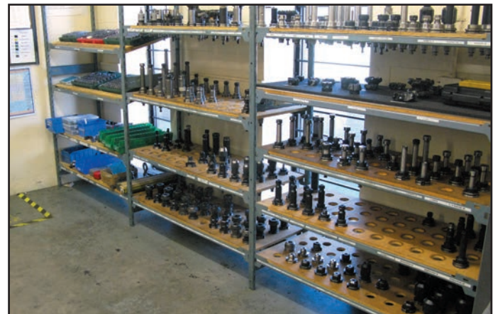
Fig. 11. Though modest in size, the Veritas manufacturing uses the latest gear and methods. Here the tool room has the different machining center tool holders already set for various machining jobs.
