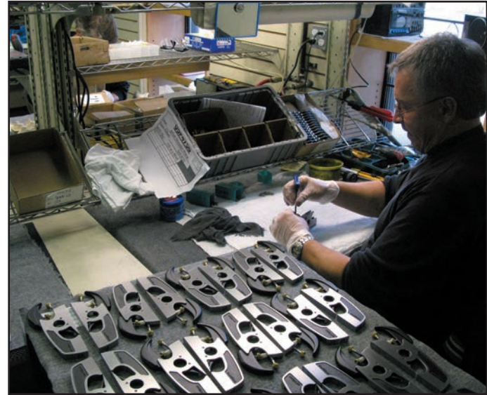
Fig. 16. In spite of all the computers, it's the human touch that does the final assembly, adjustment, and buy-off of all products. The final acceptance is not only dimensional and functional, but also visual. Marks that can't be measured can be reason for rejection.
