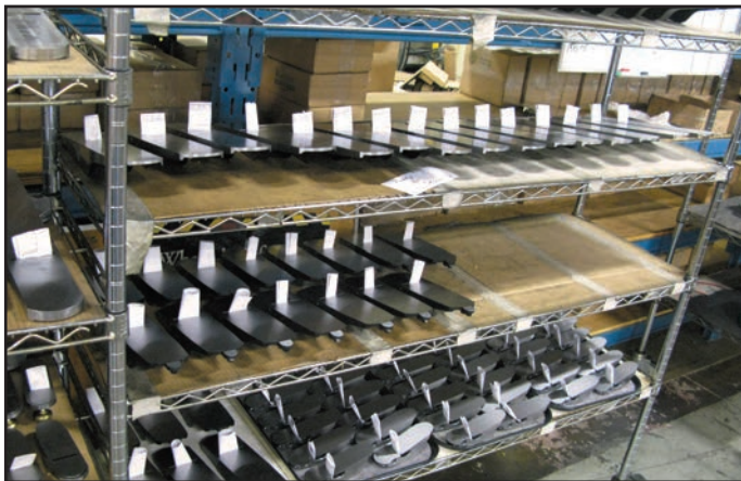
Fig. 9. Manufacturing precision parts requires careful handling. Because of the varying sizes, shapes, and fragility, material handling can range from food service carts to egg cartons.
