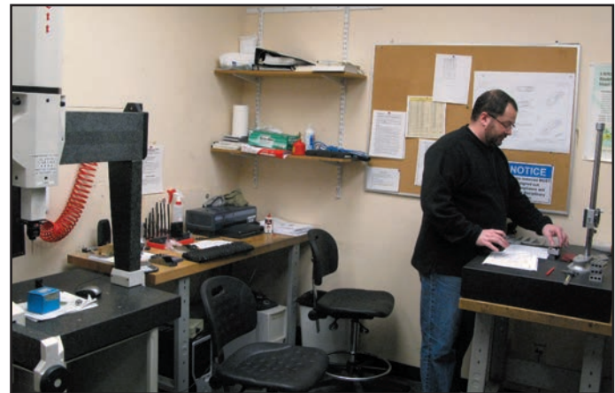
Fig. 12. Quality control is no less important when manufacturing smaller quantities. Coordinate measuring equipment is just one of the tools used in the Veritas quality process.
