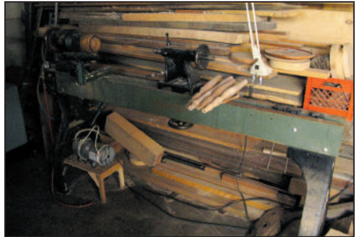
Fig. 4. This is one of the Conover lathes from the 80s. It featured floor castings, headstock, and tailstock components that the end user would purchase to make their own wooden bed lathe. It's a very flexible design from size and final configuration.
