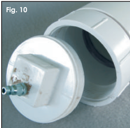
Fig. 10 To help minimize trapped bubbles in my polyester resin castings, I often immediately put them into my home-built vacuum chamber to draw them to the surface while still viscous.
