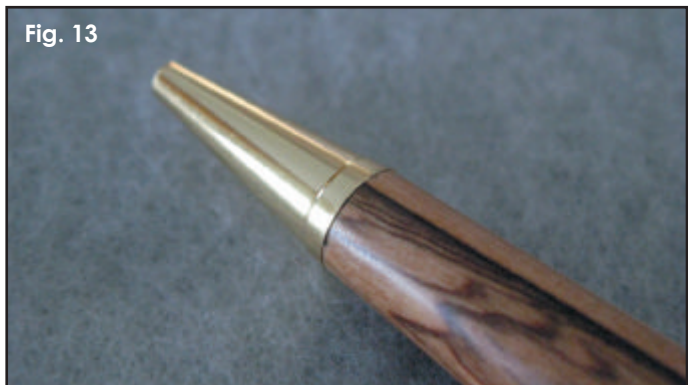
Fig. 13 These two careless mistakes on this kit pen are often found in the lower-end venues—poor fit at the nib and it still has sanding flaws.
