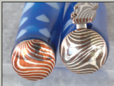
Even a winner can have some things that could be improved. The color mismatch of the crafted end caps is apparent and so is the less than optimum fit on the lower. Internal cutting had issues also.
