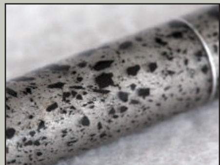
This is an interesting and well done casting, but a close look shows some of the air that was entrained in the resin, which became permanent when it couldn't be eliminated before the resin was too viscous and solidified.
