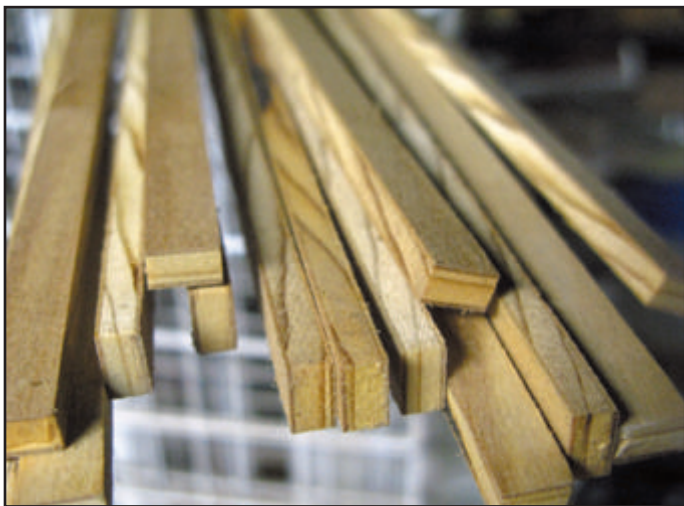
Fig. 21. Miniature stickers for drying green wood pen blanks can be homemade, and the blanks are cut generously sized and then stickered for drying.
