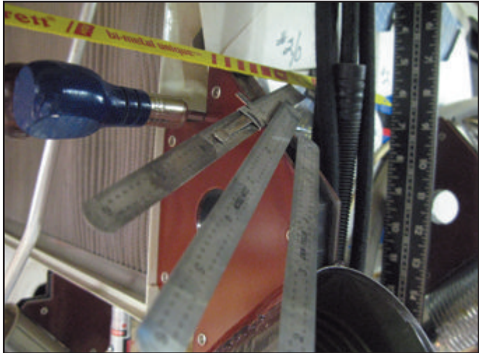
Fig. 2. Extra 6" scales, scratch awls, tin cans for pencils, and cutoff saws (yes, a hacksaw blade makes a great cutoff saw) within easy reach save time.
