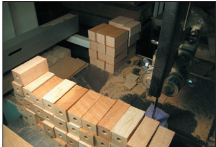
Fig. 12. Practice materials are processed for one of my classes with the drilled blanks to get tubes glued in immediately and extra blanks are cut (to remain undrilled) waiting for future needs.
