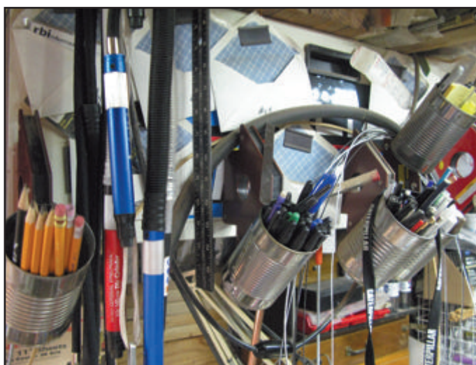
Fig. 1. Welder's magnets stuck on every metal surface allow for storage of supplies, marking and measuring items, and often-needed tools.
