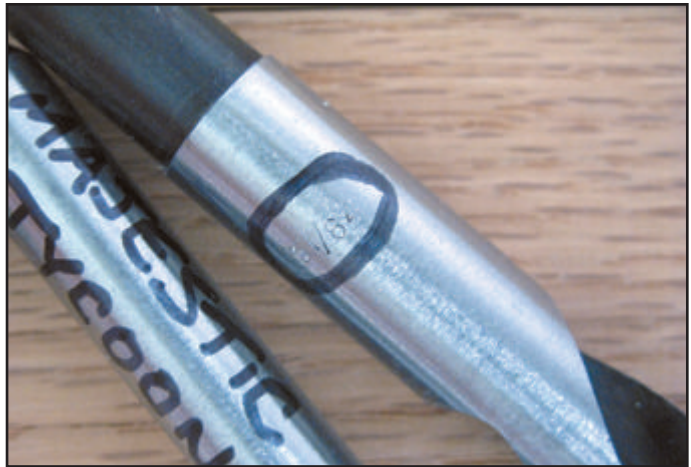
Fig. 6. Highlighting the location of the drill size makes it faster to locate—and even better, mark the kits that it is used for right on the drill.
