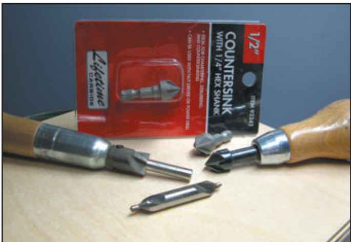
Fig. 15. Key tools for the penmaker include center drills, chamfer tools, and a handheld short pilot barrel trimmer.
