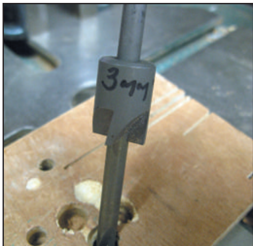
Fig. 7. If you mark the adjusting screw size on the tool, you don't need to guess whether it is English or metric, and what size it is.
