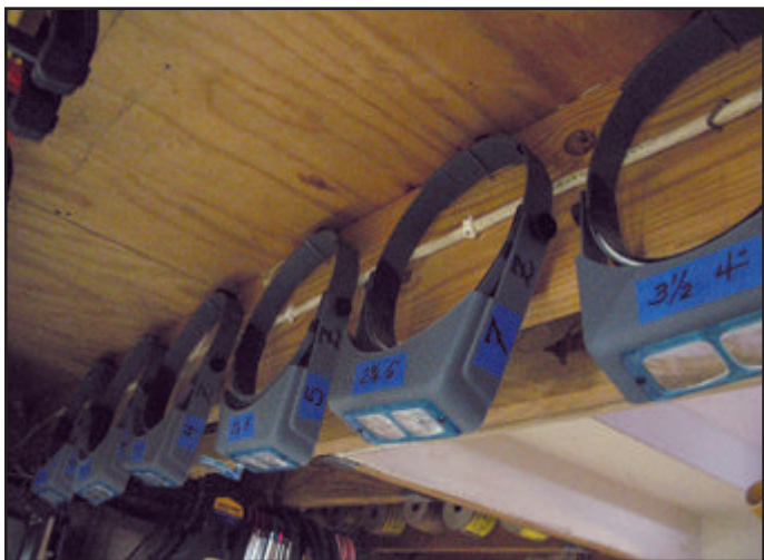
Fig. 4. If you can afford them, having a set of Optivisors (or equivalent) with the various magnifications and focal length clearly marked and readily accessible saves time.
