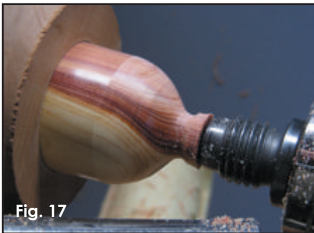
Fig. 17 The bottom is shaped still using the tailstock for as long as possible.
