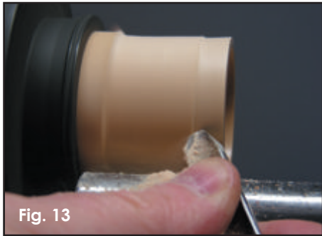
Fig. 13 The outside of the scoop body is shaped after the inside is completed.
