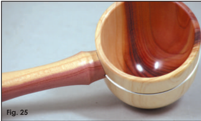
Sand the end of the handle with the bowl curve until you are satisfied with the fit.
