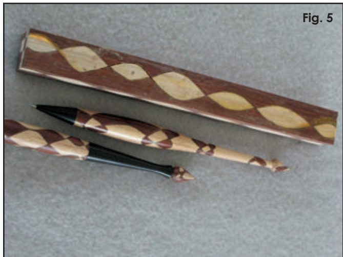
Fig. 5 The pens in the foreground began by making the glue-up shown at the top of the photo.
