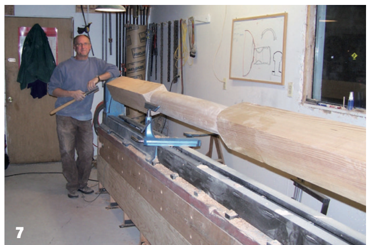
6 Production work. These 'thermed' spindles were made for a local brewery as tap handles. They were dyed black and labels affixed. The brew master told me of a conversation he heard at the bar, two patrons arguing over just how something like that can be made, one guy insisting that it was impossible to make on a lathe 7 My first long lathe, constructed out of a Vicmark long bed with an extension added, made by a local machinist firm. It allowed me to turn 12ft. As soon as I had installed this lathe I got a phone call for 15 12ft posts to be made. Divine intervention? 8 'Cog and Pawl', cocobolo, African blackwood, mahogany, brass. 6 x 6.5 x 2.5in 9 (Main picture) I work on an old Oliver tablesaw, an 88, with sliding side table and 4in depth of cut. It's a real workhorse, but wouldn't pass any sort of European safety standards! 10 Box elder burl and holly, ring box 11 Madrone ring box 12 Walnut ring box 13 European pear ring box
