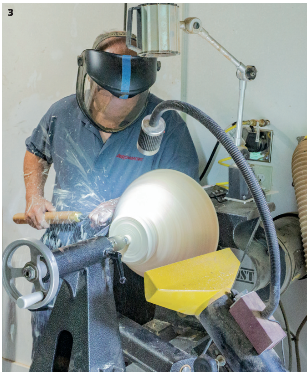
1 A good starting point for lathe height is when the elbow joint is at the same height as the centreline of the spindle. Be certain you are standing on your anti-fatigue mat(s) 2 I find that I need two mats to provide the necessary support. Notice that the 2X4 height shims are lagged only to the lathe. Nothing is attached directly to the floor 3 Take your time creeping up or down on the correct height. Once found, you may be able to spend more time at the lathe with less aches and pains
