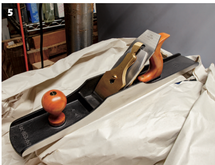
4 I use Naval Jelly to remove any rust that has already occurred and use Boeshield T9 as the rust preventative for cast iron and steels in the shop that are susceptible 5 I use T9 on the woodworking tools in my shop. Planes and in particular the irons need protection in my shop 6 I return my less frequently used planes to their original box. I find it helps provide protection from rust, nicks and dings, and helps them being easily found
