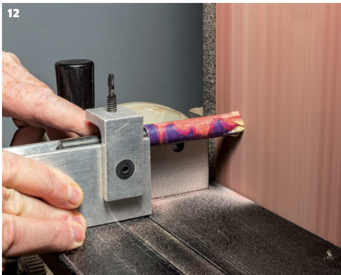
12 Getting good results, the face of trimmed wood and brass tube perpendicular to the tube ID requires that the platen and fence be trued perpendicular to the belt
