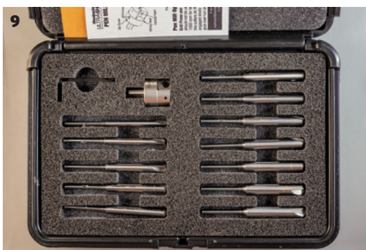
3 Part of my stable of barrel trimmers. I modify them based on my needs and often use tape to create a low-tech bushing for a good fit inside the brass tube 4 Reasonable speeds and feeds will help maintain the life of a barrel trimmer. It is easy to overheat them and ruin any finer cutting capabilities 5 The goal of a barrel trimmer is to trim the wood flush with the brass tube. Good placement and gluing will help to minimise the amount needing to be trimmed 6 If you don't have a set of modestly priced diamond hones in your kit, I suggest you add them. Ideal for touching up barrel trimmers, skewers, parting tools, bedans, and others 7 Exactly the WRONG way to touch up a barrel trimmer. Do you think you can touch up all four edges remaining at the correct angle and keep all edges coplanar? 8 Far easier to touch up the cutting edges, remaining in contact, and maintaining coplanarity of the cutters. Like tools, keeping them sharp is easier than sharpening 9 A recently released barrel trimmer family. A single cutter head with two carbide cutters mounted accepts any one of the pilot diameters available in the kit 10 My favourite feature is the amount of 'overhang' the cutter has with the brass tube. This prevents the brass tube from creeping between the cutter and the pilot 11 If you trim laser cut kits, a barrel trimmer usually breaks things. Having a fixture to pilot the blank on the brass tube ID works great, whether homemade or store bought
