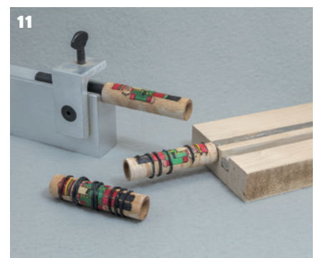
3 Part of my stable of barrel trimmers. I modify them based on my needs and often use tape to create a low-tech bushing for a good fit inside the brass tube 4 Reasonable speeds and feeds will help maintain the life of a barrel trimmer. It is easy to overheat them and ruin any finer cutting capabilities 5 The goal of a barrel trimmer is to trim the wood flush with the brass tube. Good placement and gluing will help to minimise the amount needing to be trimmed 6 If you don't have a set of modestly priced diamond hones in your kit, I suggest you add them. Ideal for touching up barrel trimmers, skewers, parting tools, bedans, and others 7 Exactly the WRONG way to touch up a barrel trimmer. Do you think you can touch up all four edges remaining at the correct angle and keep all edges coplanar? 8 Far easier to touch up the cutting edges, remaining in contact, and maintaining coplanarity of the cutters. Like tools, keeping them sharp is easier than sharpening 9 A recently released barrel trimmer family. A single cutter head with two carbide cutters mounted accepts any one of the pilot diameters available in the kit 10 My favourite feature is the amount of 'overhang' the cutter has with the brass tube. This prevents the brass tube from creeping between the cutter and the pilot 11 If you trim laser cut kits, a barrel trimmer usually breaks things. Having a fixture to pilot the blank on the brass tube ID works great, whether homemade or store bought
