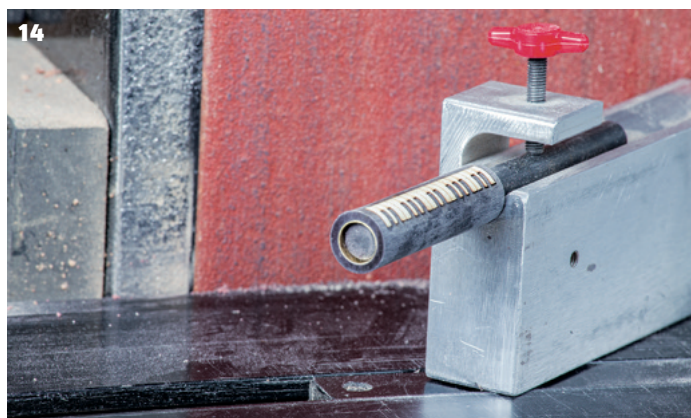
14 Whether homemade or store bought, a good sanding fixture will support the blank to almost the very end, allowing for accurate results
