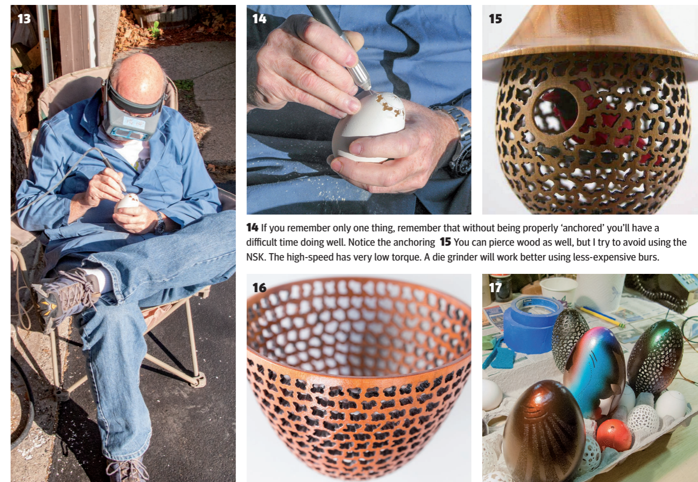
13 A key to good piercing is stability. Plenty of light, a comfortable chair, PPE, and elbows being well supported.
