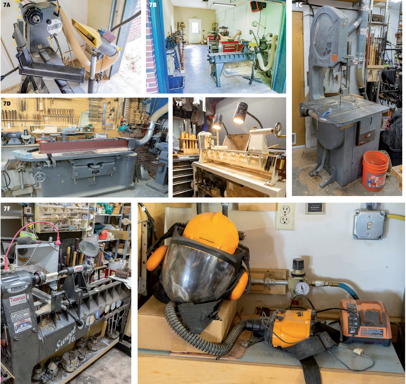
7 Plumbing your dust collector hose to the location where you are generating the dust is an effective way to reduce what is thrown in the air to ultimately get breathed 8 Regardless of your dust collector and shop system, never ignore the fact that effective PPE on your head or face is a wise idea
