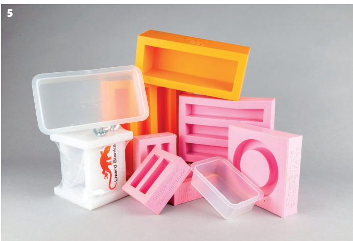
3 Aluminium foil cuts away so easily, I never waste time removing it prior to turning on the lathe. 4 What size blank do you need? You can make any size you want with no investment but pennies-worth of aluminium foil. 5 Just some of my moulds. These, my purchased moulds, and my 'on-demand' create my own foil moulds, and let me cast any resin material we hobbyists might use in any size desired. 6 When I'm casting pen blanks, I use the desired size blank as the pattern to fold my foil around when making the mould
