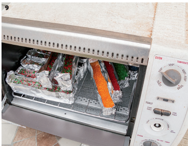
7 Foil pen blank moulds want to bow out in the middle. An easy way to support the side walls of pen blank moulds while casting. 8 The silicone mould works great but only does one size. Can you see the infinite flexibility of using the foil mould idea for diameter, wall sizing, and depth of casting for any application size? 9 I usually post mould bake my polyester resin castings. Not required but it reduces tackiness of the outside of the blank. Done outside in an old, shop only, toaster oven at minimum temp. 10 Ready for cutting and drilling. Foil left on until it gets turned away on the lathe. Notice the cut marks, interface indication, and blank matching. Just a good habit regardless of material
