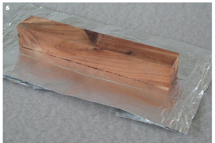
3 Aluminium foil cuts away so easily, I never waste time removing it prior to turning on the lathe. 4 What size blank do you need? You can make any size you want with no investment but pennies-worth of aluminium foil. 5 Just some of my moulds. These, my purchased moulds, and my 'on-demand' create my own foil moulds, and let me cast any resin material we hobbyists might use in any size desired. 6 When I'm casting pen blanks, I use the desired size blank as the pattern to fold my foil around when making the mould
