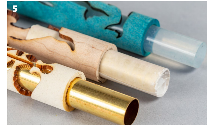
5 Rather than use the raw brass tube as your depth control device, wrap it in waxed paper or use the available silicone assembly dowel
