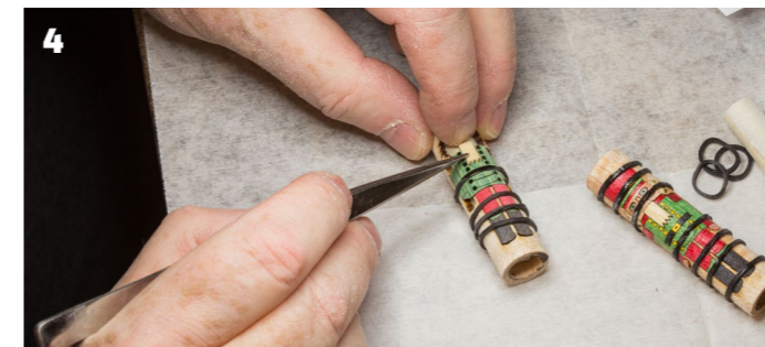
3 A key to success is having the component parts flush to the inner diameter so they can be adhesively bonded to the brass tube when it is time. 4 With pieces of different species and needed clearances for assembly, there are spaces. Position the pieces visually, equalising spaces
