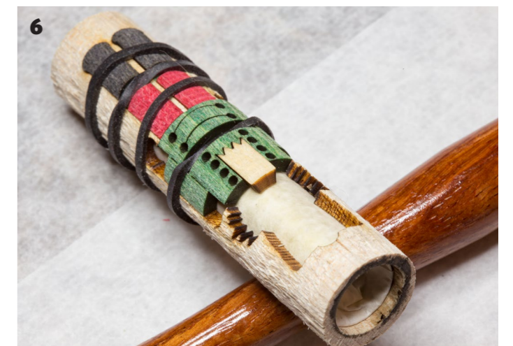
6 Lightly tack the pieces in place with CA as you go. Use the provided rubber bands to help position and hold the pieces as needed
