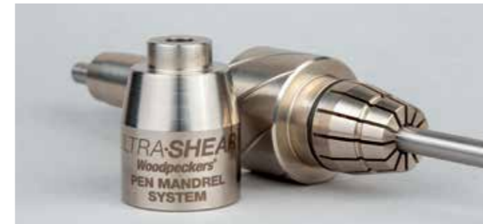
The No.2 MT mandrel saving function revolving tailcentre uses ABEC1 bearings, is CNC machined 303 stainless steel with a 12-jaw collet clamp compression controlled by a mandrel saving nose piece
