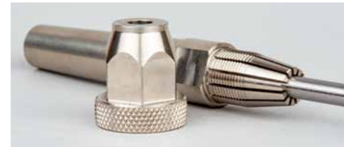
The headstock clamp, a CNC machined 303 stainless steel with a No.2 Morse taper, a 12-jaw collet clamp and a threaded knurled compression nut with wrench flats
