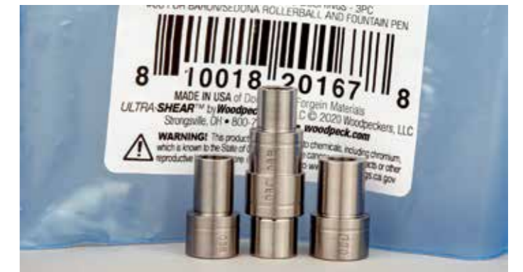
Each package of bushings indicates the kits that the bushings are designed for. Notice the C(ap) and B(arrel) markings added to the bushing numbers to indicate orientation
