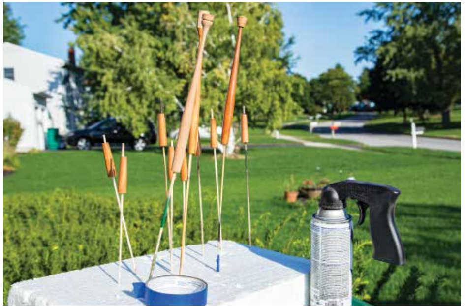
Doing a lacquer finish on pens. Outdoors with plenty of ventilation is my choice. Notice the pistol grip on the rattle can of lacquer
