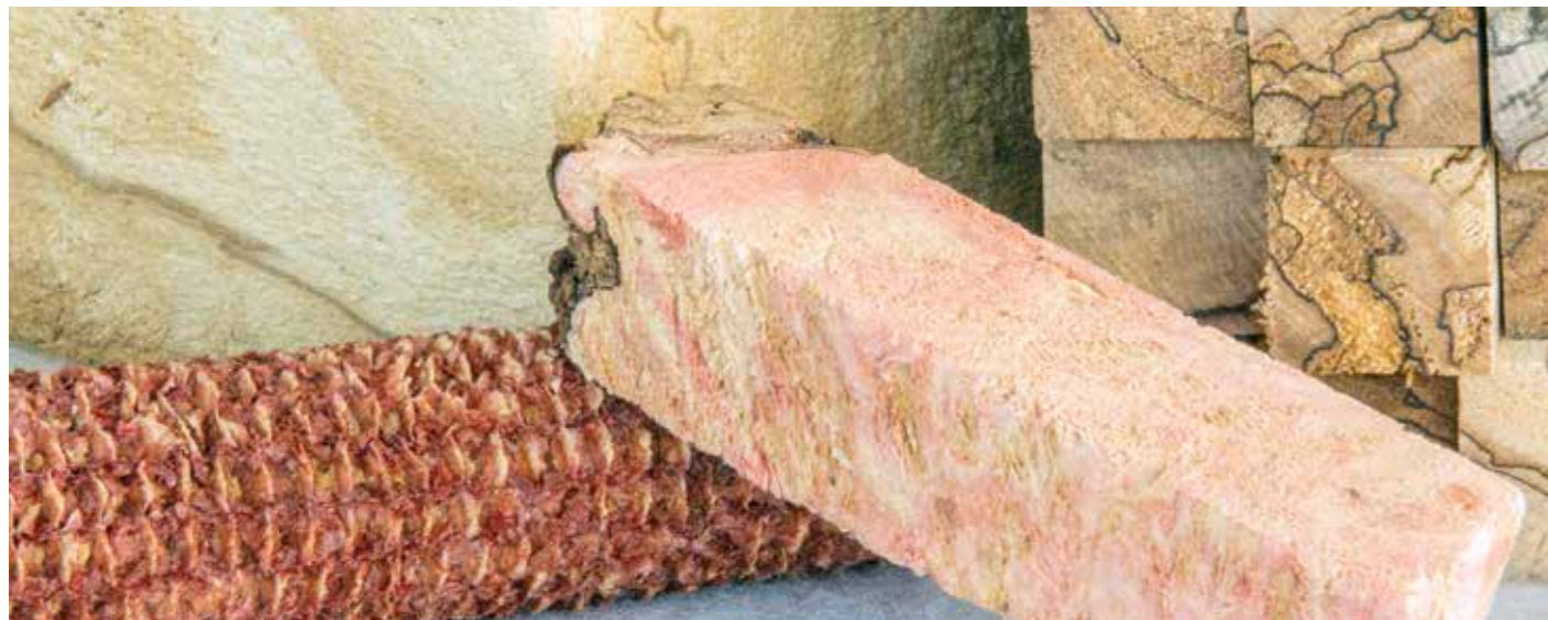
Dense woods require no stabilisation. Porous or punky woods do. If you can't tell visually, a thumbnail pressed into the timber will tell you
