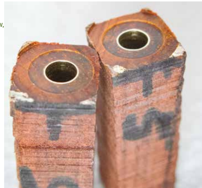
Pen blanks with a tube glued in and faced ready for turning
