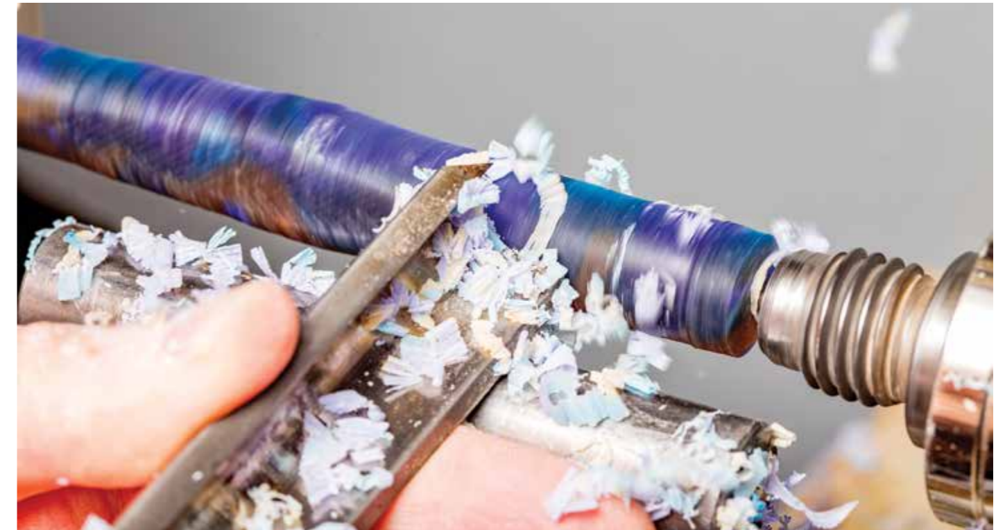
A properly sharpened and presented HS tool will cut any acrylic I've encountered. Carbides work as well with high speed and light touch
