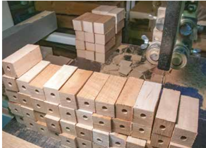
Bandsawn pen blanks ready for tube insertion
