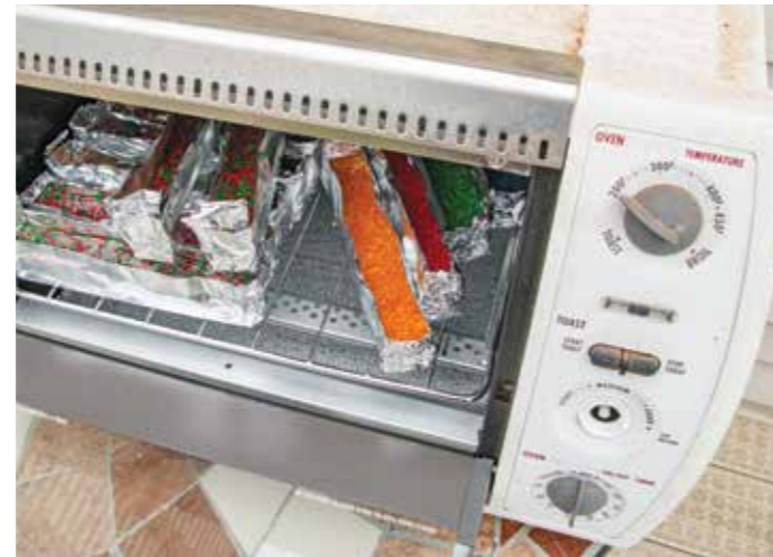
Use a shop dedicated oven or microwave for drying wood and baking castings
