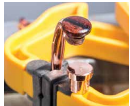
The wooden end cap will work exactly as the pressed cap when properly glued in under some compression
