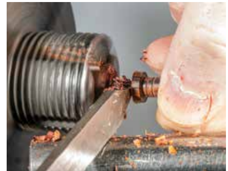
Size the head of the end cap based on your application and part it off for reverse mounting
