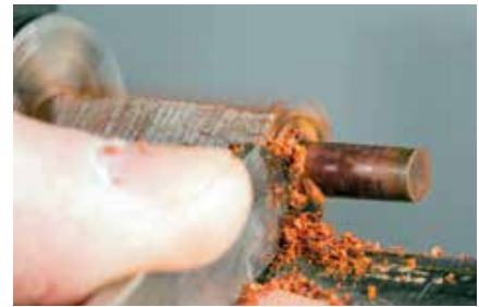
Use the same process for sizing and removing the radius from the inner corner on the nib
