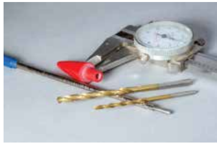
The two drill bits for nibs are the same for virtually every Cross style ink-fill. Using 3.175mm and 2.03mm works well
