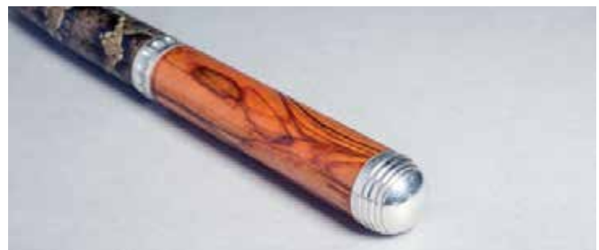
As metal is easily turned on your lathe, aluminium can be made into caps, nibs, and trim
