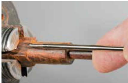
Plan your nib length before you get too far. Mark for drill depths and end point
