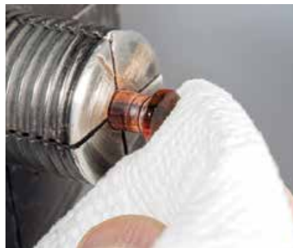
Add your finish to the end cap. I tend to use a CA finish for ease of application and durability
