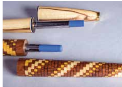
Press depth is very forgiving with the 7mm kit. As long as the brass portion of the transmission seats, all is OK
