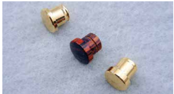
End caps have no issues with grain or orientation so feel free to use nearly anything
