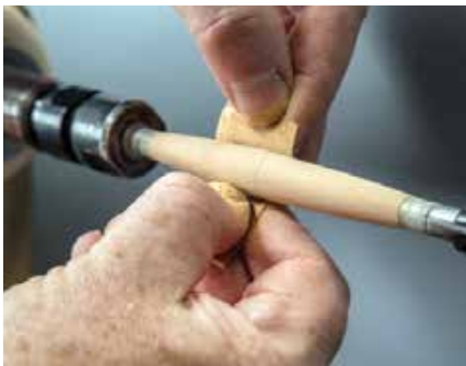
Butting the two barrels together makes it easy to have them fit perfectly since you create them simultaneously
