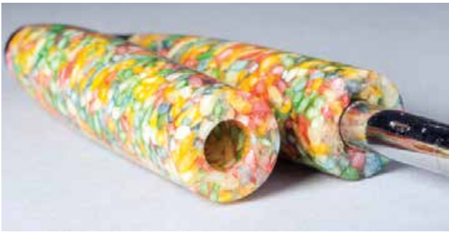
You can make up any missing length by leaving some of the interface barrels unsupported by brass
