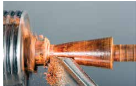
Shape the nib with the tool of your choice, being aware that there are drillings inside
