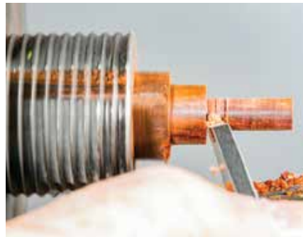
Add some glue traps as well and be certain there is no radius in the corner to prevent flush assembly
