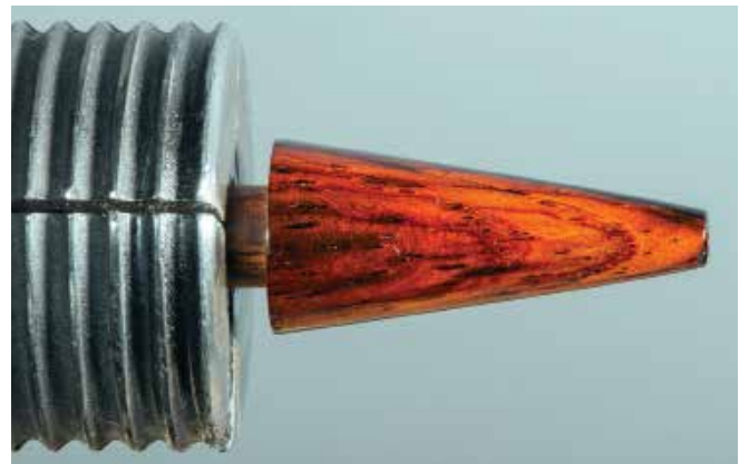
Sand through the grits until you are content with the shape and finish. Again, I use a CA finish
