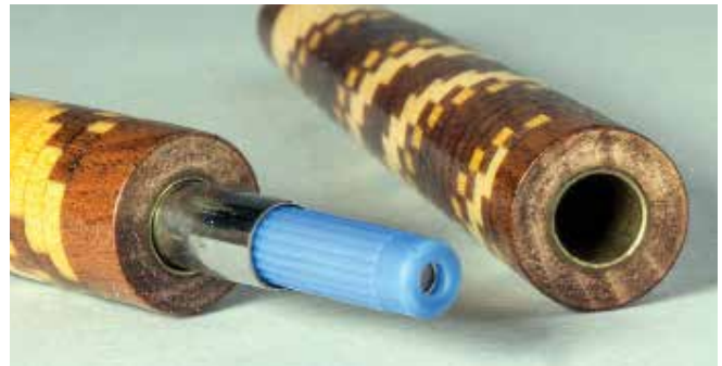
When the situation dictates, you can also insert another brass tube and trim as needed
