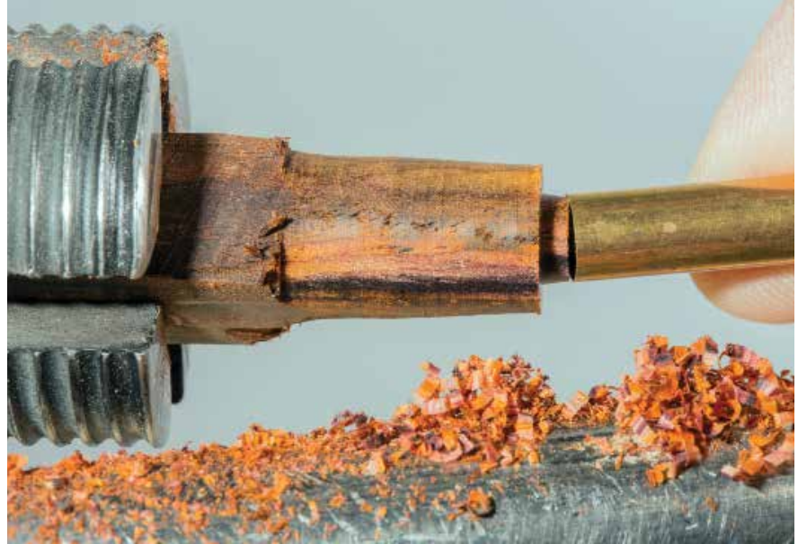
Use a brass tube to size your shaft on your end cap. Quick, easy, and no measurement errors
