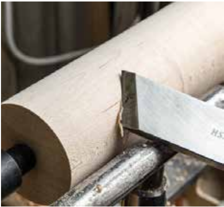
Rest a bit high, tool at 45°, bevel rubbing then clear, sharp edge, and it will cut curls rotating by hand
