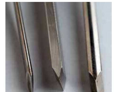
Some skews come with the corners 'broken'. You may need to do this to your skew for easy toolrest sliding
