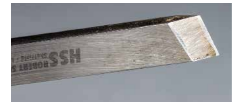
Grind surfaces aren't parallel or the cutting edge isn't dead centre? A sharp cutting edge works
