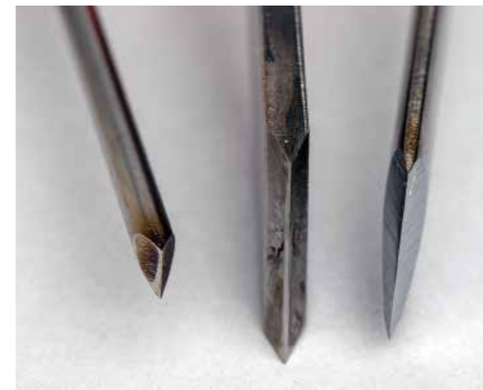
The most common cross-section skews are rectangular, oval, and round. Round are usually home-made
