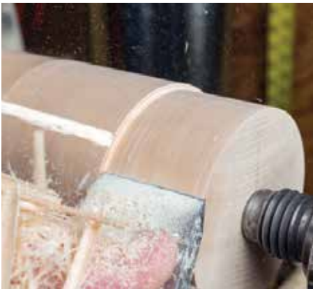
Tool flat on the rest, edge parallel to the axis, rub the bevel and slowly lift the handle
