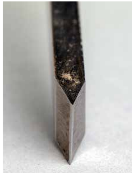
I use a bench grinder for a hollow grind on my skews letting me touch them up with a diamond hone
