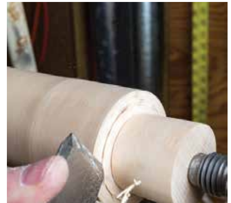
The end grain cut works superbly to clean up torn grain. Take thin sections at a time for best results
