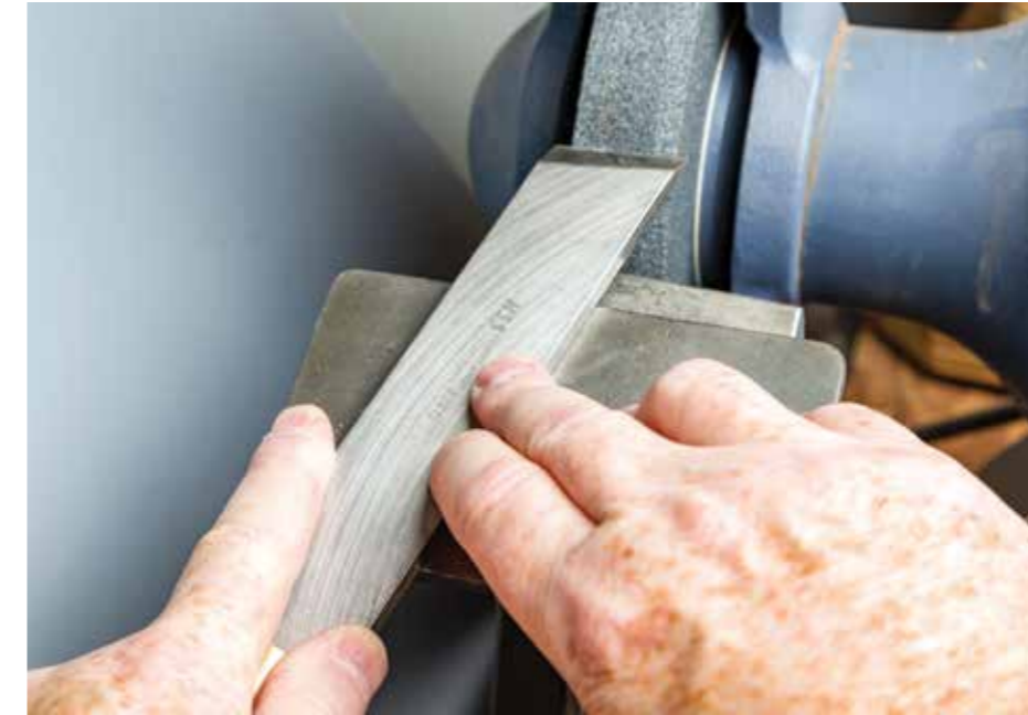
Adjust to the desired angle. Slide the tool up the rest to contact the wheel parallel to the edge
