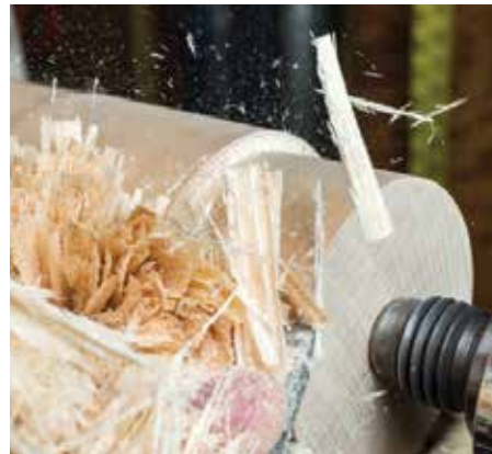
As the diameter decreases, follow it right down as you would with a parting tool
