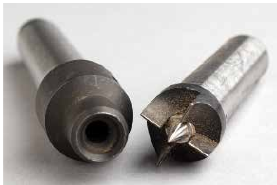
Rather than the standard four spur, pick up a safety or cup centre. With or without the pin, it will aid your learning
