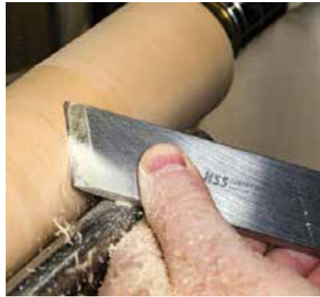
The skew excels at the planing cut. Stay in the sweet spot with a sharp tool and light touch
