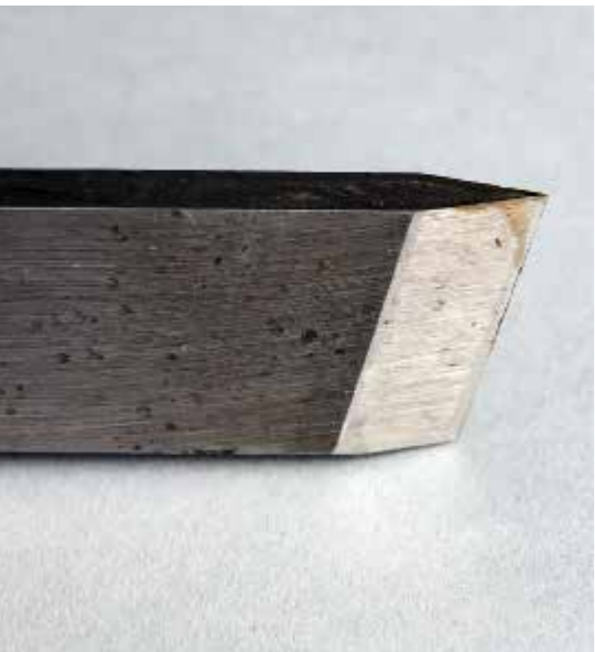
You may opt for a flat grind based on your sharpening system. The Sorby ProEdge and other belts create this
