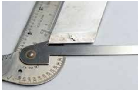
All of my skews fall in the 70° range although I eyeball them when grinding rather than measure
