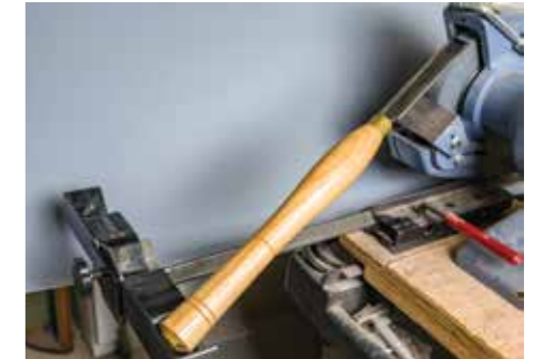
The skew jig attachment to the Wolverine makes sharpening quick and easy
