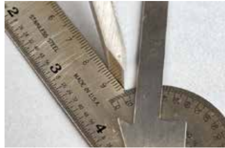
My included angles vary, but my go-to skew for detailing is right around 40°. A good general purpose angle
