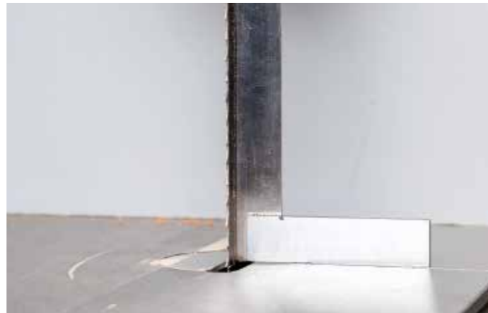
Use a square to ensure that your bandsaw table is truly perpendicular to the blade
