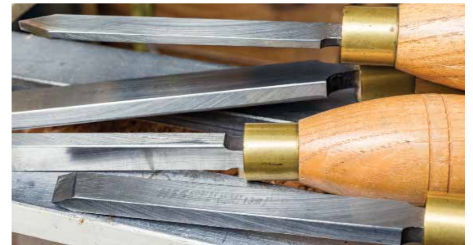
Break the sharp corners on all of the tool shaft corners that will come in contact with your toolrest
