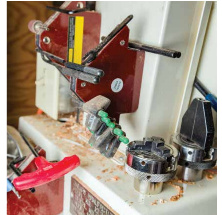
Welder's layup magnets work well to keep the needed drills, wrenches and other metal items at hand
