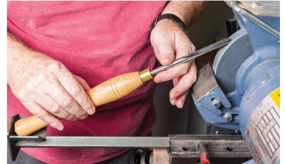
If you took the time to set up the jig, why not touch up the tool before returning it to the rack?
