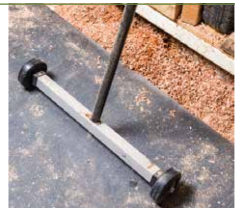
One of my handiest gadgets. A strong magnetic bar 'broom' on rollers to find dropped metal items among the chips
