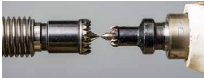
Not perfect, but it is the best I can do on my main lathe. Align the centres of your lathe using the KISS test between your headstock and tailstock
