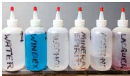
Decanting my commonly used solvents makes them handy to keep nearby and precisely dispense as they are needed
