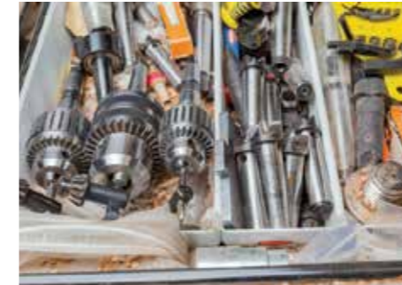
I keep the keys to the drill chucks hand tightened in the jaws of the proper chuck
