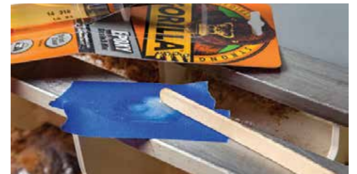
Just one of the many uses for painter's tape. A couple of strips lets you mix adhesives anywhere with an easy clean up
