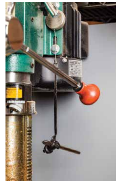
My retractable chuck key mechanism on my drillpress is a convenience, but also a safety feature
