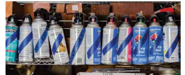
Marking the colour on open spray cans makes finding the correct colour much faster in my workshop
