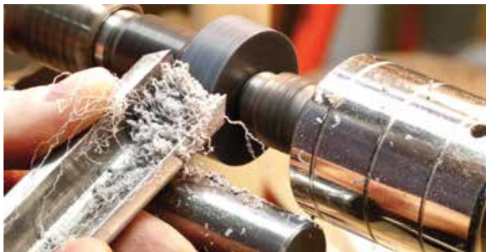
Being a filled plastic, Corian cuts extremely well with woodturning tools
