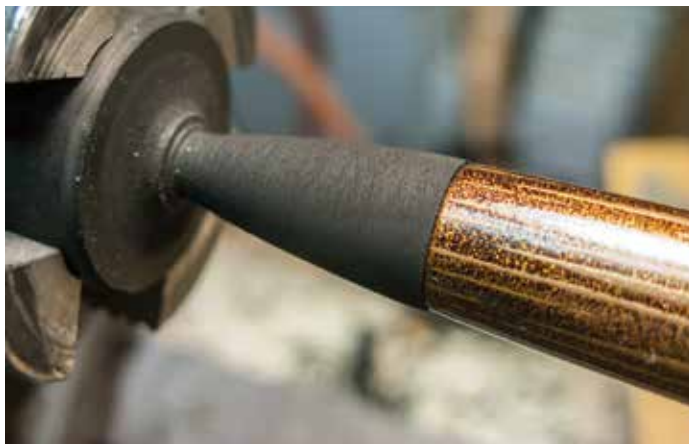
A test fit for a custom nib blank prior to separation for finish cuts and sanding
