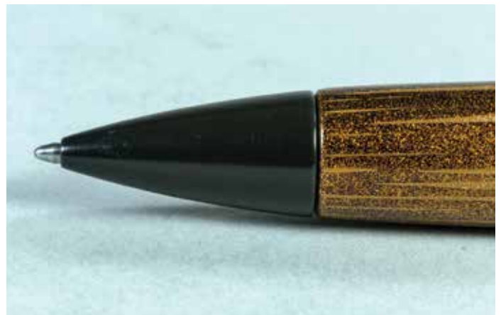
Final dry fit prior to finish sanding and then MicroMesh to get the ebonite to pop
