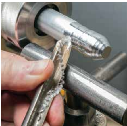
A sharp, properly presented tool will deal with brass, aluminums, bronze and soft steels (alloy depending)
