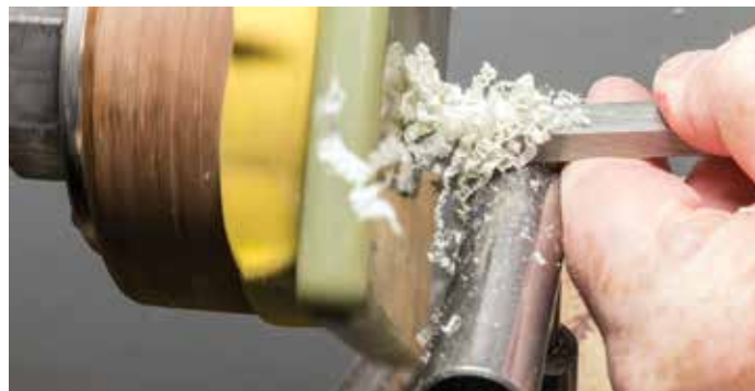
Hollowing and dishing tend to work better with a scraper. The aspect ratio of the material will have an impact on your choice
