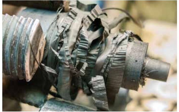
Depending on your speeds and feeds, you can slice the stuff like tape to remove stock quickly
