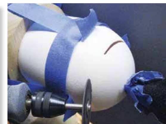
Low-tack painter's tape has a variety of applications from masking off areas for protection to padding to low strength holding needs
