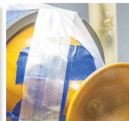
Lightly padded with low-tack painter's tape in the jaws, this turning is secured in the chuck with fibreglass-reinforced tape for the light work done on the foot
