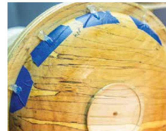
A platter needing some light sanding is fastened to a faceplate platen with hot melt glue. The painter's tape provides an easy removal without tearing out grain
