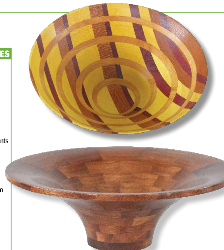
A bowl turned from glued-up flat stock fastened together with wood glue. The glue bond strength even with this very thin wall is exceptional
