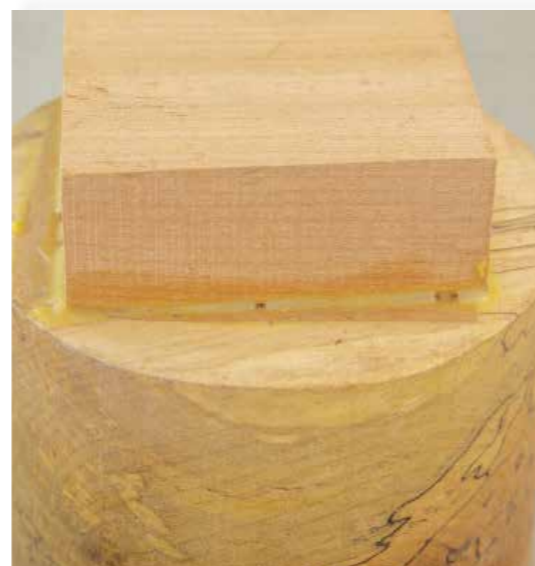
A common use for wood glue in turning is to add a high-strength glue block to fasten a faceplate. Grocery bag paper is added to the joint to allow for cleaving
