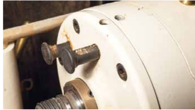
The engagement pins on my lathe represent two different measurement methods. While sturdy and well built, it is good practice to not stress the locking mechanism
