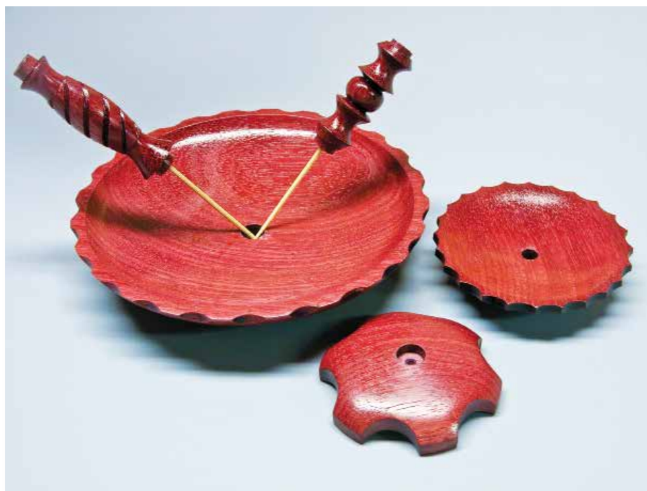
When there is no need for precision, parts can be indexed as needed for sanding, grinding or other processing. The candy dish rim scallops sanded with an air die grinder
