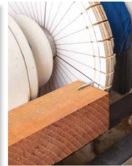
The indexing wheel has holes or slots for whatever 'latching' mechanism you use. Double-sided tape holds the wood block in place with the nail located on top of the block
