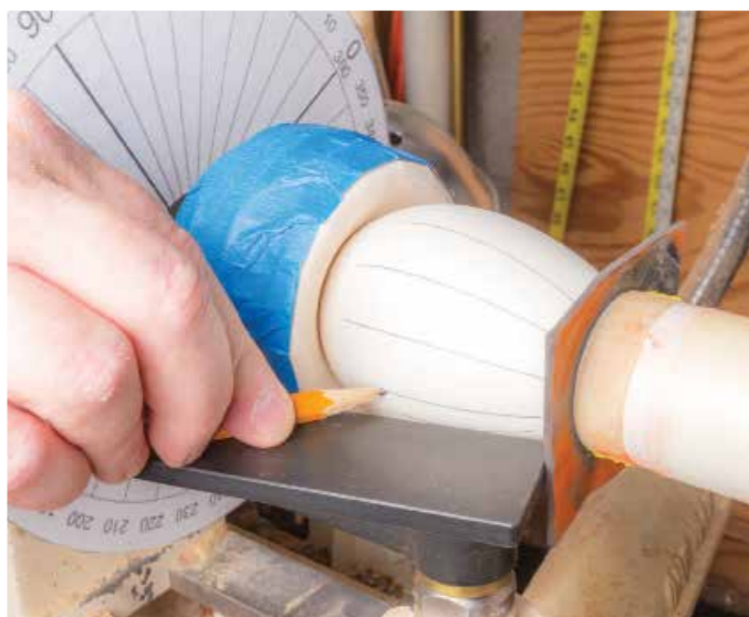
While many of the indexing systems will support the use of tools and cutters, I favour using the indexing system to do marking. Once marked, the heavier work is done without stressing the lock
