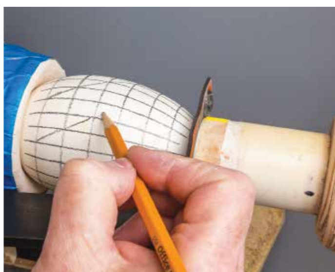
Adding the axial marking at proper positions along with the already available radial marking opens new opportunities. An entire spectrum of precision spirals can now be explored
