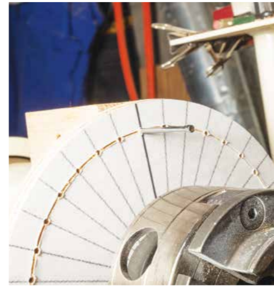
A tool cut to assist locating the drill makes the plywood and paper indexing system easy to make and certainly inexpensive. A nail and a hole in a wooden block complete the system
