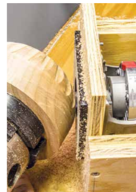
There is a host of tools that can be brought to bear on turnings while they are mounted and indexed on the lathe. From the router article, a bowl being scalloped on the outside
