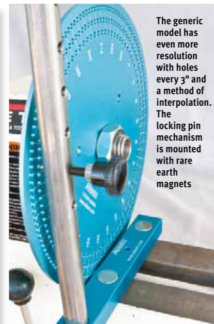
The locking pin mechanism mounts to existing hardware and provides precision locating and locking. The rotation is broken into 72 positions or 5°
