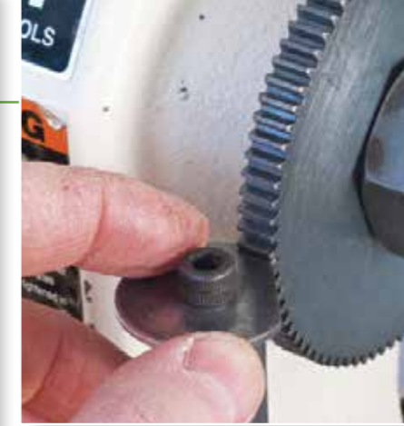
Rotating the washer from the ground flat to the original outer diameter locks this indexing system in position. Far stronger than needed but made from scrap parts
