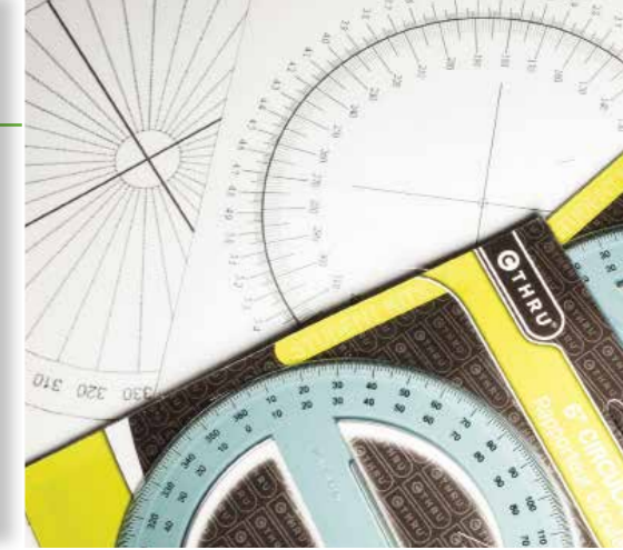
Your home-made indexing system can be built around a protractor glued to a board or a computer print, attached to a board with spray adhesive
