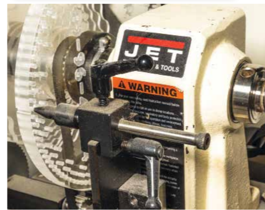
The indexing wheel can be mounted on the inboard or outboard side of the headstock spindle. The locking pin arrangements vary from quite simple to complex
