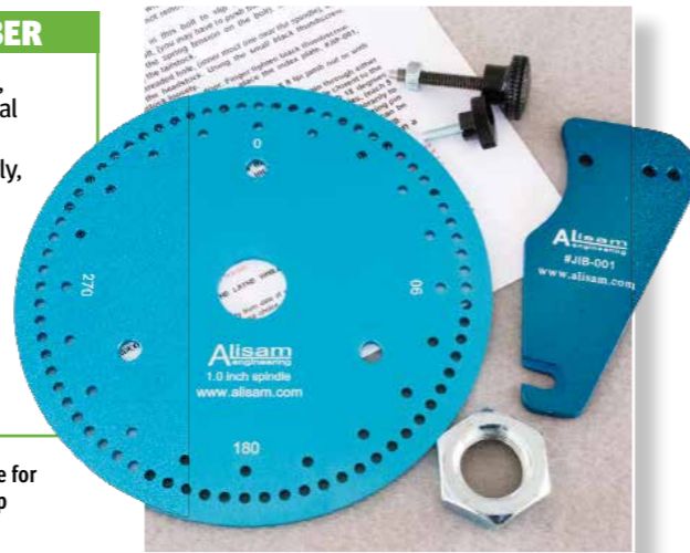
The generic model has even more resolution with holes every 3° and a method of interpolation. The locking pin mechanism is mounted with rare earth magnets
