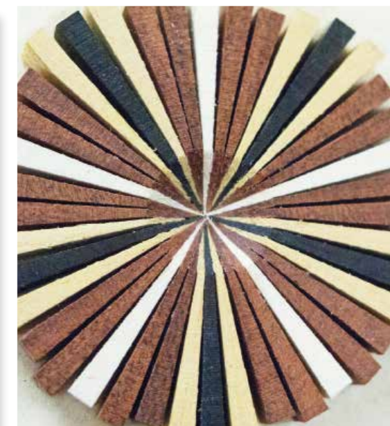
The beginnings of a glue up of an open segmented hollow form. The indexing plays a key part in the precision needed for a successful open segmented turning
