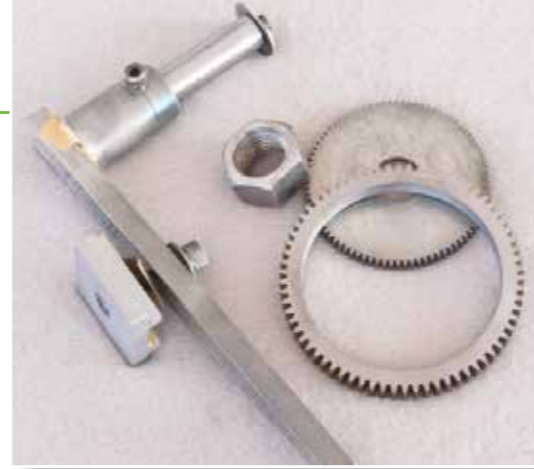
Depending on your skills and the equipment available, you can work with a variety of materials. A reclaimed gear and some metal parts silver soldered make the indexing system
