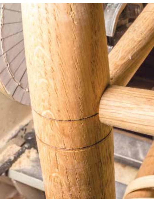
Drilling spindles at precise angles is now very easy. Whether 90° or some other angle, the spindle can be marked for drilling or simply drilled when positioned
