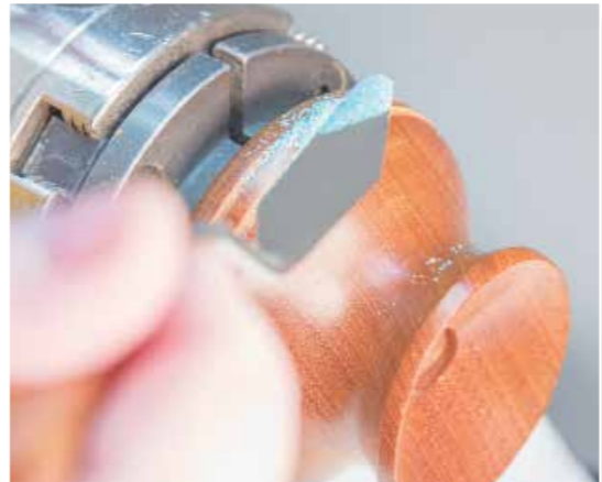
An artist's palette knife works nicely to deposit the granules into the channel on the top of the turning. Use a catch paper on the bed to recover the costly powders spilled
