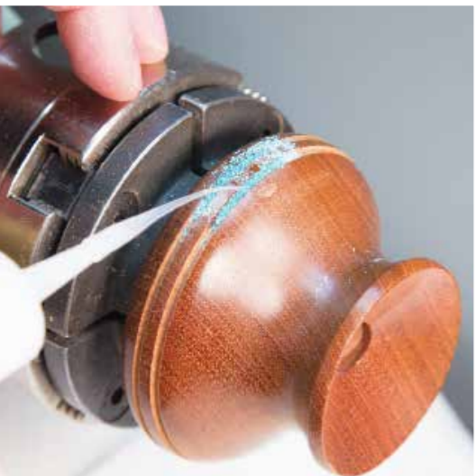
Dispense very thin CA adhesive to solidify the granules in place. Leave a working area without adhesive to continue after rotating for the next area
