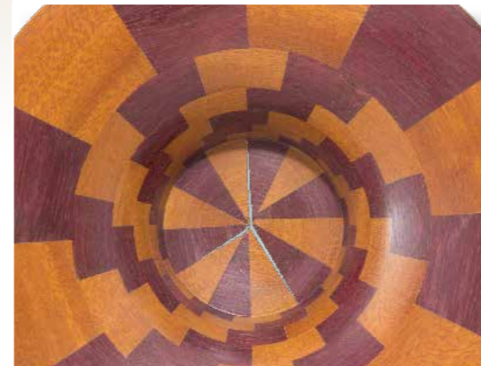
A problem area for many segmented turners is the bottom. Because of the geometries, end grain glue joints and expansion rates, failures are common
