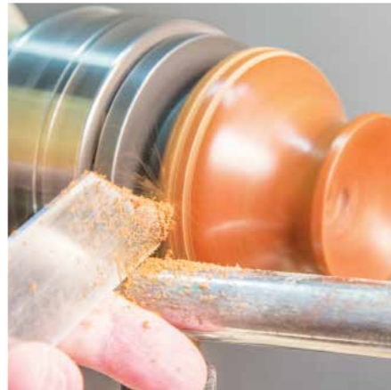
A pocket to receive the dry particles is created in one of a variety of ways. Here the parting tool is used to create parallel channels to be filled with turquoise
