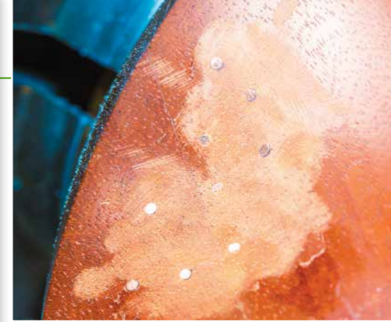
File until flush and then move to abrasives. All of the turning and rough sanding is done prior to precious metal addition so final finish sanding is all that is required
