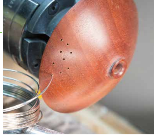
Drill your desired holes with only about 0.06mm clearance. This will allow sufficient adhesive to be wicked into place
