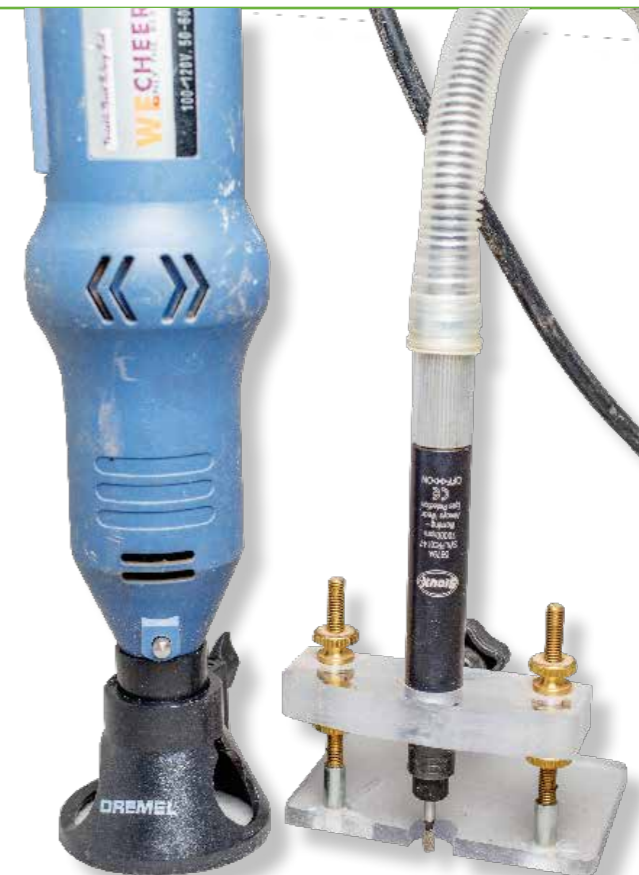
Handy tools for inlay, especially for flat areas. The depth base for the Dremel style tools makes tracing much easier. A die grinder with a luthier's base is also a welcome tool when inlaying
