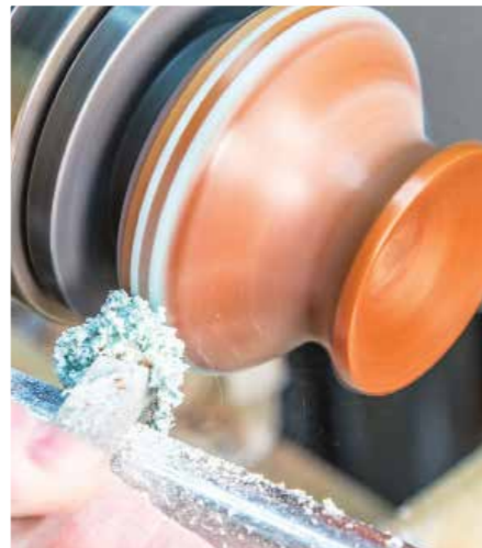
After completing the deposition and hardening of all of the materials in all of the channels, the stone or metals are cut back to level. A scraping cut with carbide cutters works well
