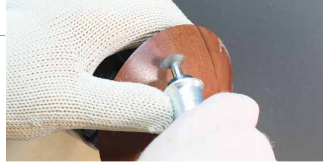
Safety items should certainly include eyes and nose protection, but don't forget the chemical resistant gloves. Here, a Kevlar carving glove offers protection when using a power carver
