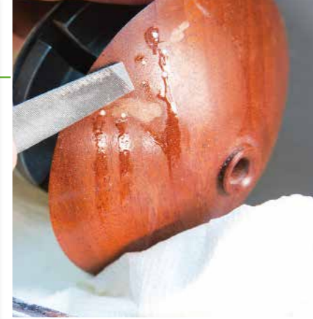
Clip the wire close to the surface and then bond in place using thin CA adhesive. The small clearance will wick in the CA and cure quickly
