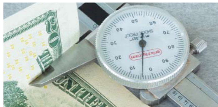
You can use typing bond paper, tin foil, tape, playing cards, or even currency to shim things as needed. Just for reference, currency and typing paper are in the .004in range
