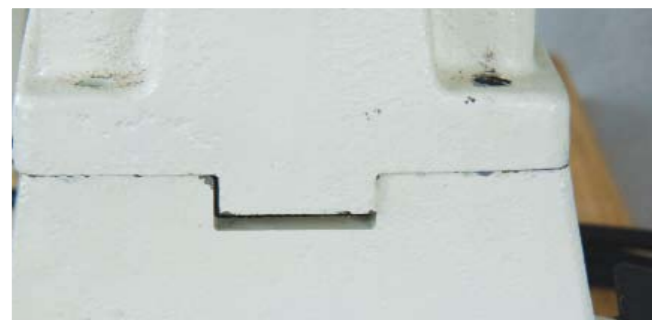
The gap in the bed usually allows sufficient adjustment for the alignment in that plane. If you need more, a file judiciously applied to the casting of the base of the headstock may help
