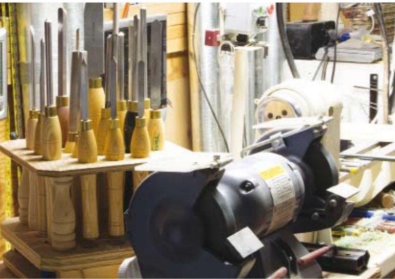
Usually stationed immediately to the left of my lathe, this roller rack holds my grinder and tool rack at a convenient height and position. The tool rack is homebuilt with scraps and a lazy susan roller base
