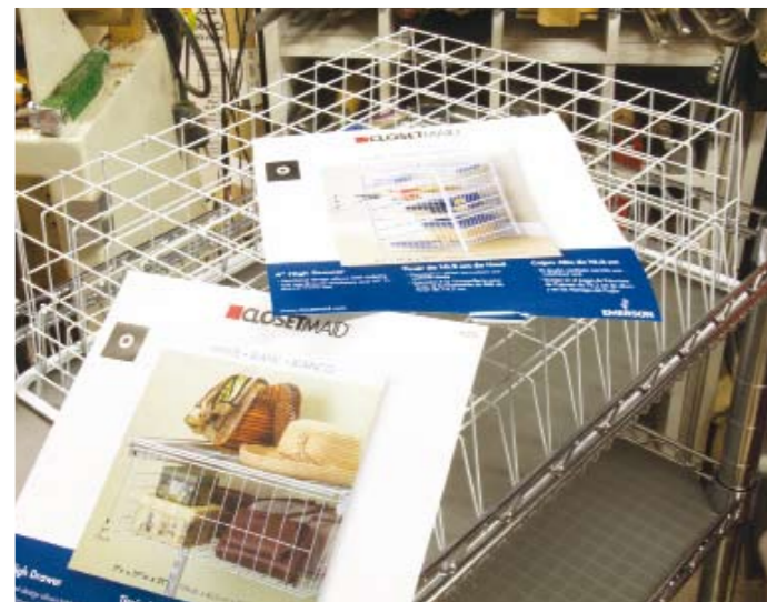
A simple idea for tool storage. Two closet storage racks purchased at the local home improvement centre. One deep and one shallow. Fastened together and used upside down, they make a great tool holder
