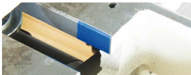
I favour using tape where possible. I want it to stay in place as I am reassembling things after shimming as needed. You can use nearly anything you have at hand to keep things spaced properly
