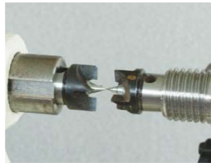
You can also use a couple of spur centres to do your alignment. It is important that the tips not only meet but that the axis of both headstock and tailstock tapers are in line
