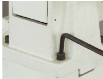
Nearly all of the common lathes available today are held in alignment with the headstock mounting bolts. The days of pinning equipment in alignment are long gone
