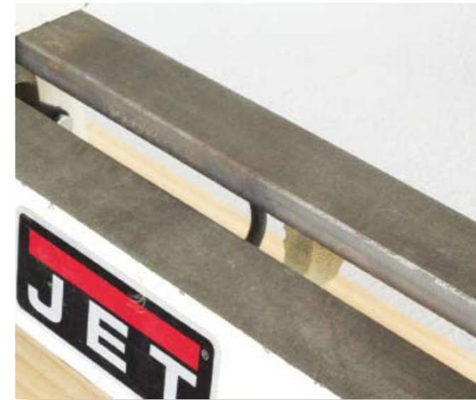
Waxing the ways of the lathe is counter-productive. It makes you put excessive clamp load on the banjo and tailstock to prevent slipping. A slight amount of surface rust is actually desirable. The slightly rusted surface makes slipping a non-issue
