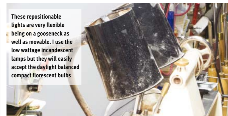
Not a major expense or difficult task, add sufficient lighting directly overhead to supplement workshop or natural lighting as needed. Colour temperature is optional but I find daylight balanced less fatiguing
