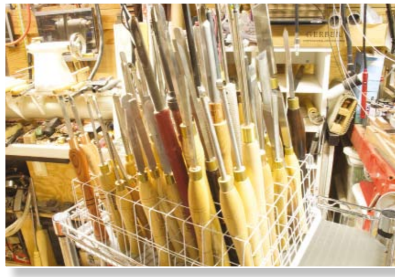
Located on a food service roller cart, this tool rack makes finding the desired tool an easy task. The two racks were fastened together with four screws to hold them together. If you think that having the points up is dangerous, use a tiered carousal with the cutting edges pointing down
