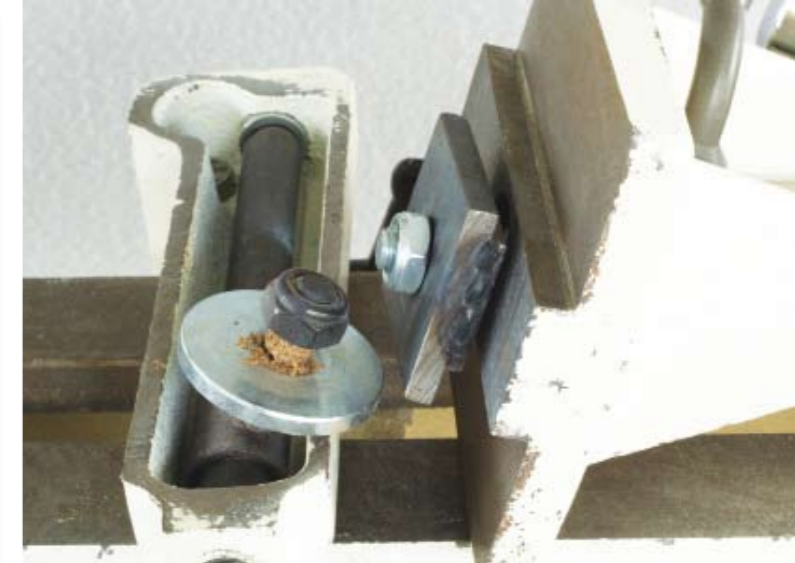
Which do you think works better to clamp things? Obviously the plated washer on the left is easier and less expensive to provide. Make or have your shop handy friends make up some replacements like that on the right
