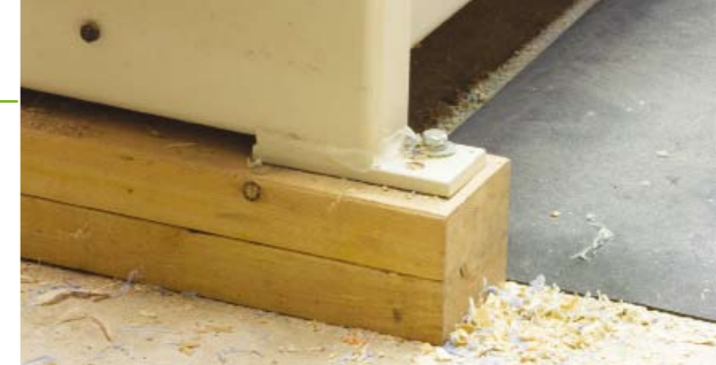
Creep up on your ideal height always using your intended anti-fatigue mat. Once you've found it, don't rely on shims. Make your lathe height durable and lasting. The lathe isn't lagged to the floor but is securely fastened to the correct height blocks
