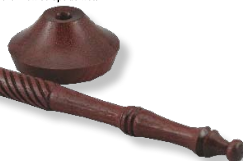
From the trimmings and pen blank from the original purpleheart block. A single piece pen using some kit parts. The four quadrants of the base glue up are not easily seen until close examination and are even pleasing then
