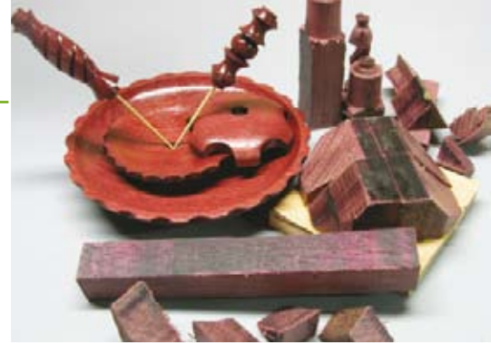
The major pieces all cut from the 50 x 50 x 150mm block of purpleheart. All of the pieces for the creation turned and finished except the finial. You can see the planned glue up scraps for the pen stand, pen blank, and finial stock. A few scraps as well
