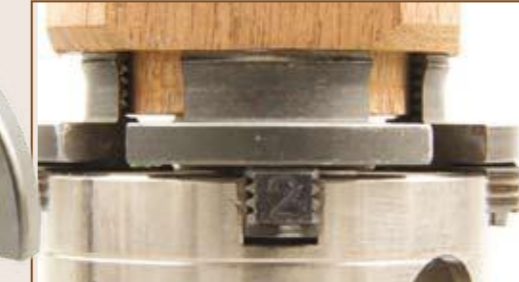
ABOVE: Mounting for best accuracy and safety requires that the work rest on the top jaw surface is cut appropriately for the jaw style and in contact with the jaws, yet isn't touching the bottom of the jaws
