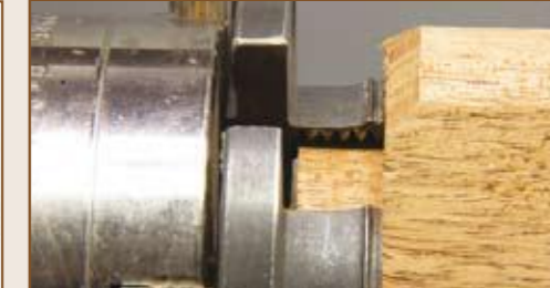
ABOVE: With maximum jaw engagement, referencing to the work from the top jaw edge, and the 'daylight' completely underneath the work you can be assured of the most concentric mounting possible
