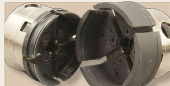
ABOVE: Even within the size range and functionality, there are options to select from based on your particular type of turning. This brand of No.3 jaws are available in the standard and deep depth
