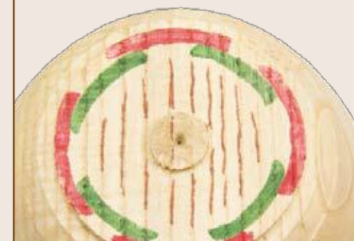
ABOVE: With maximum jaw engagement, referencing to the work from the top jaw edge, and the 'daylight' completely underneath the work you can be assured of the most concentric mounting possible
