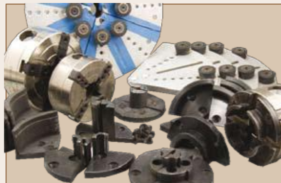
ABOVE: Once the manufacturer and service range has been selected, there is a wide range of optional jaws available. Jaws are not usually interchangeable among manufacturers
