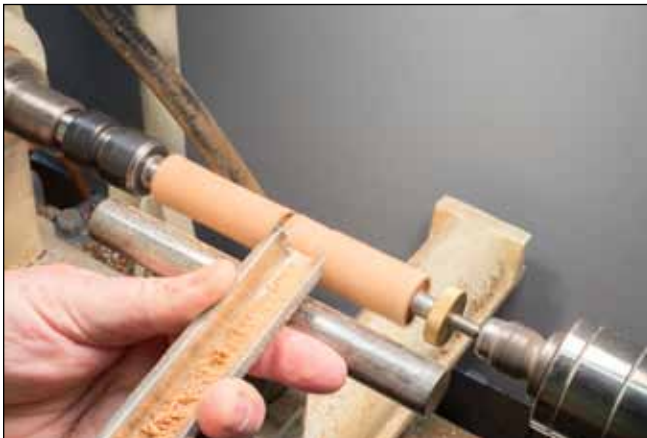
16 Pens can be turned with almost any tool; one of the best for the task is a spindle roughing gouge.
