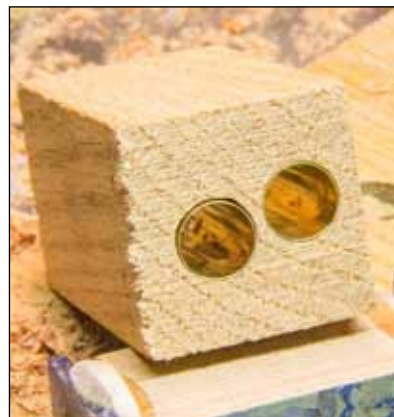
6 Proper sized holes with good gluing surfaces, left, require sensible speeds and feeds. Slower is better than too fast. Overheating the material or burnishing the hole, right, will cause inaccurate sizing or poor gluing.
