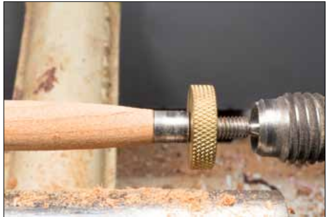
17 Turn and sand right to the bushing dimension at the ends of all of the 7mm pen barrels.
