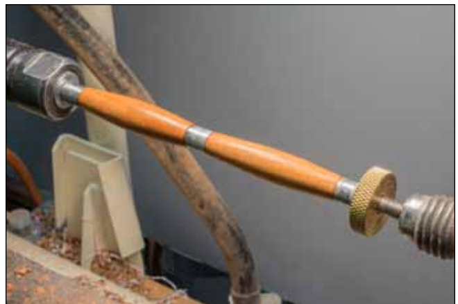
19 Almost any finish can be used on pens. Friction finishes are fast and easy for starters.
