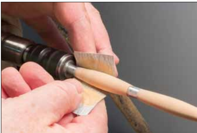
18 Even with the simple 7mm kit, sanding on the mandrel can create a pleasant flowing shape.
