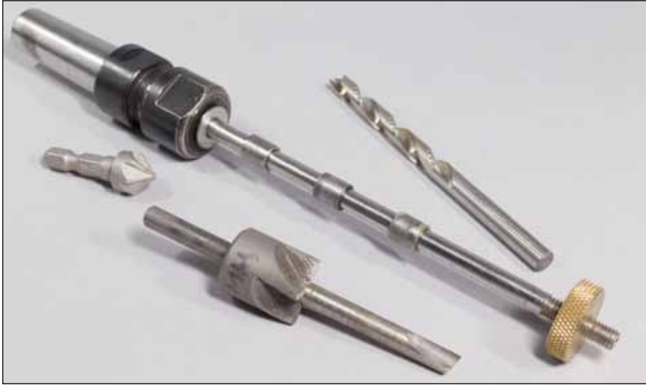
5 These are the special tools needed for basic pen turning, from left: mandrel with bushings, chamfer tool, pen mill, and properly sized drill bit.
