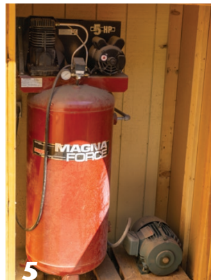
5 To keep the shop noise down and conserve space, this compressor and phase converter are located in a small enclosure outside the shop.
