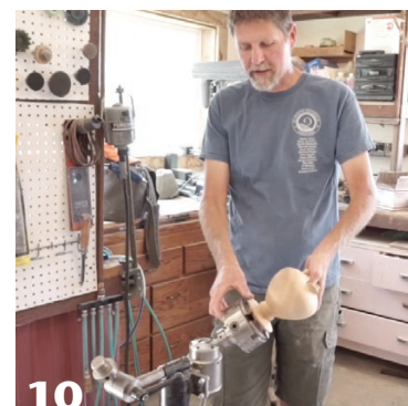
10 In a separate teaching area, students have access to adjustable workholding stands used when carving, piercing, or otherwise embellishing work after it has been turned.
