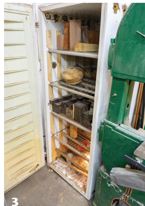
An old freezer has been repurposed as a wood drying and storage cabinet, with the addition of a low-wattage light bulb and vents.
