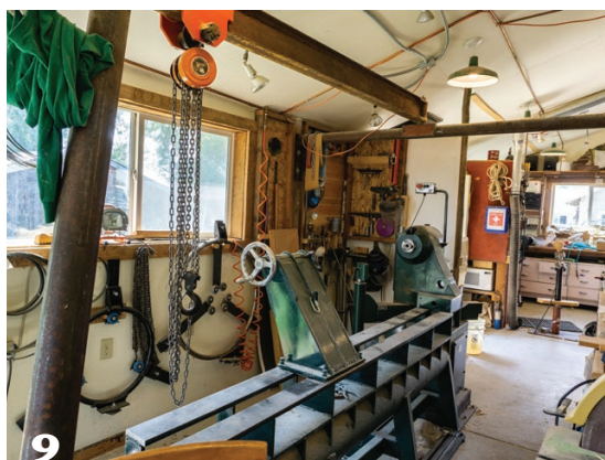
9 Because Trent's personal work often requires large blanks, his overhead lift system is capable of handling pieces up to two tons.
