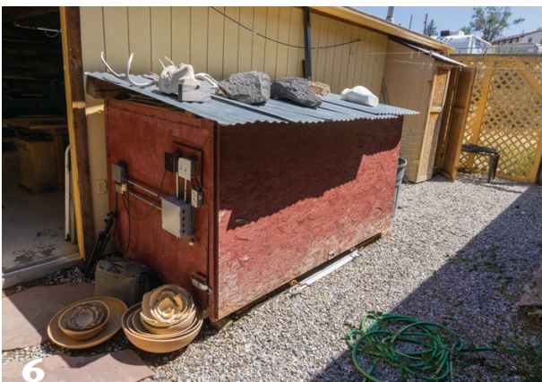
6 Keith's drying box is located outside and has controls to set and maintain a temperature and humidity for drying.
