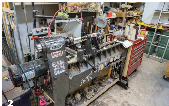
This lathe is used for spindle work and is self-contained with compressed air, vacuum hood, task lighting, chucks, tools, and measuring equipment.
