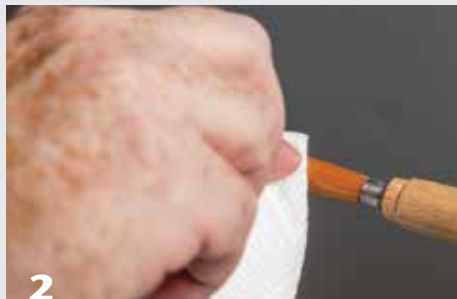
1 Wet a corner of a folded paper towel, without puddling, to prepare for the CA application. Rotating the work by hand, use the wetted towel to "paint" one complete coat on axially, end to end, around once.
