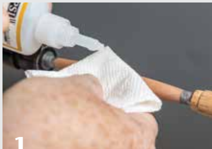
1 Wet a corner of a folded paper towel, without puddling, to prepare for the CA application. Rotating the work by hand, use the wetted towel to "paint" one complete coat on axially, end to end, around once.
