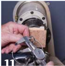
Use a caliper to transfer the desired ring size to the wood.
