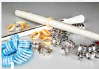
1 A set of ring gauges is helpful for determining either the size of an existing ring known to fit or a previously undetermined ring size.
