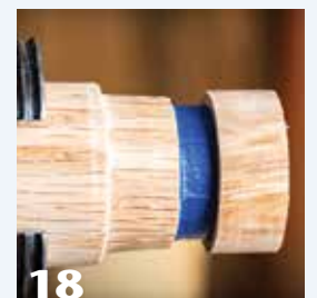
To work on the outside diameter, a shopmade mandrel is useful. Turn a spigot to accept the ring.
