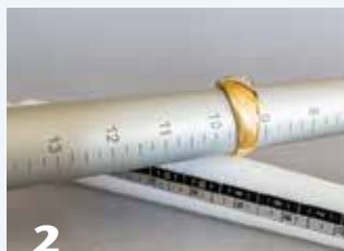
1 A set of ring gauges is helpful for determining either the size of an existing ring known to fit or a previously undetermined ring size.
