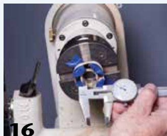
To fine-tune the inside diameter, the author sands away material using sandpaper wrapped around a dowel. Stop the lathe and check progress using a caliper.
