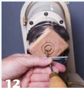
The author turns the inside and outside diameters with a parting tool.
