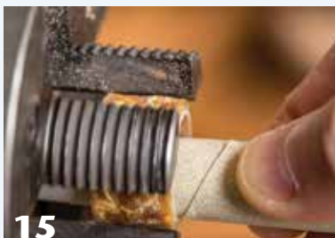
To fine-tune the inside diameter, the author sands away material using sandpaper wrapped around a dowel. Stop the lathe and check progress using a caliper.
